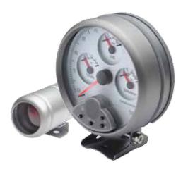
This four function gauge is used as a tachometer (0-10,000 RPM), voltmeter (8-16V), oil pressure gauge (0-100 PSI) and water temperature gauge (105F-250F) all in one. The housing color is black/titanium, and also comes with a shift light accessory and with 7 different illumination colour combinations.
